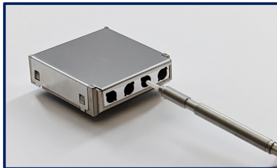
Terminus shown installed into a COTSWORKS RCP™
