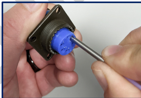
Examples show Lightly installed into COTSWORKS RCP and 38999 style connector.
