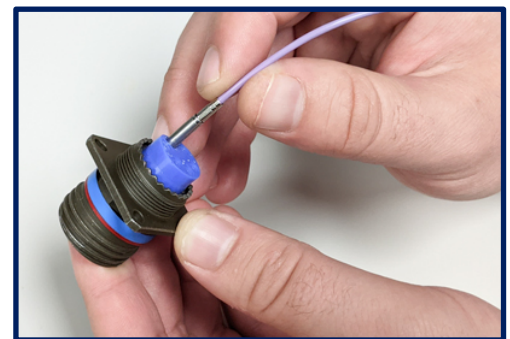
Examples show Lightly installed into COTSWORKS RCP and 38999 style connector.
