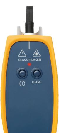
A non-programmable, battery-powered device with an On/Off button and limited modulation control.
