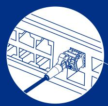
SFP form factor defined by MSA standards INF-8074i and SFF-8431. The compact size makes it easier to install into a switch and test vs. a large handheld VFL device.
