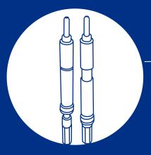
Rear-mounted cylinder compresses to release terminus with spring-actuated return once inserted, eliminating the need for M81969/1-03 insertion/removal tool.
